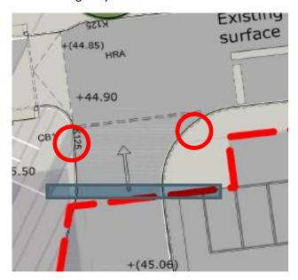
**Recommendation:** Provide appropriate tactile paving across this access. Any tactile paving used should where possible, have a colour contrast with the surrounding materials.
