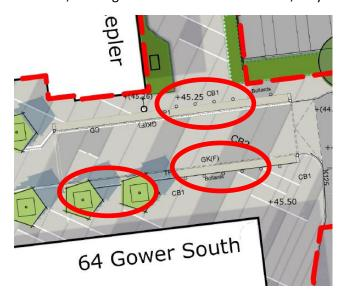
**Recommendation:** Rationalise the number of the number of bollards to ensure the main desire line remains clear of obstructions. Shorten the length of tactile paving so that it extends as far as the first street tree on the south side of the crossing. A short depth of corduroy warning paving could be provided on the kerb line of the remainder of the flush section on the north and south side to warn the visually impaired of the presence of the carriageway.
